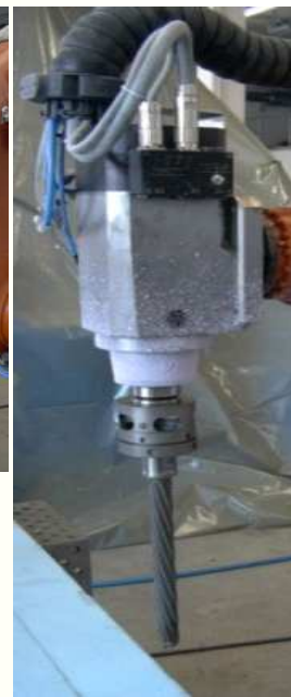
Hollow spindle and extraction for polystyrene cutting
