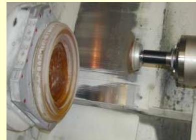
Grinding spindle 20000 rpm , 15 kw
