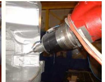
12 kw, 24000 rpm plug in spindle
