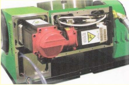
Compact units with built in drive motors fully protected by pressurisation.
