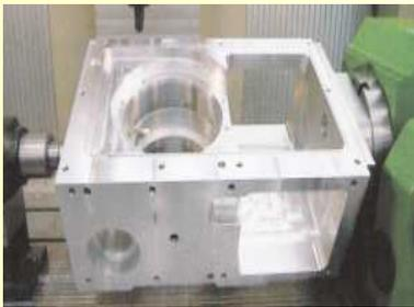
High mechanical strength derived from monoblock construction from special alloy.
